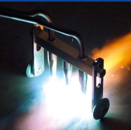
Flammrichten Flame Straightening
